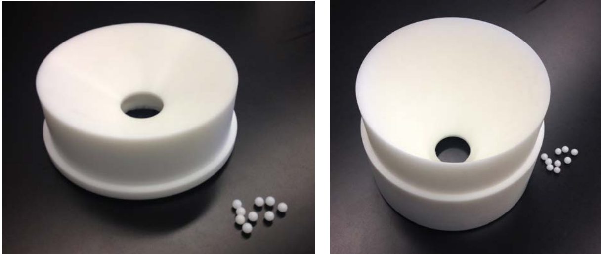
Figure 2-38. Machined cones with 30 (left) and 60-degree (right) hopper angles.
