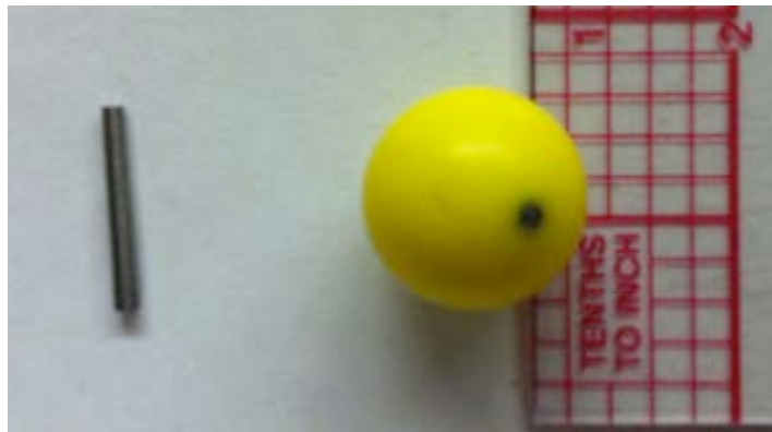
Figure 1-24. Prototype 12.5 mm diameter polyethylene pebble with tapered stainless steel pin insert.
